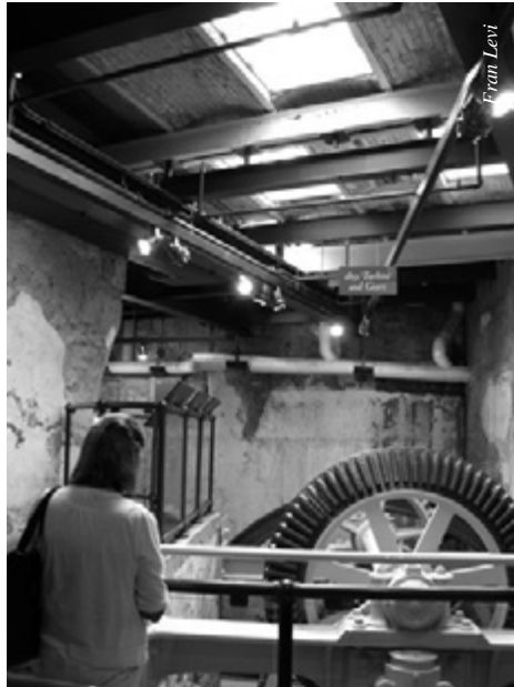
Turbine and gears installed in 1851 are in their original location.
