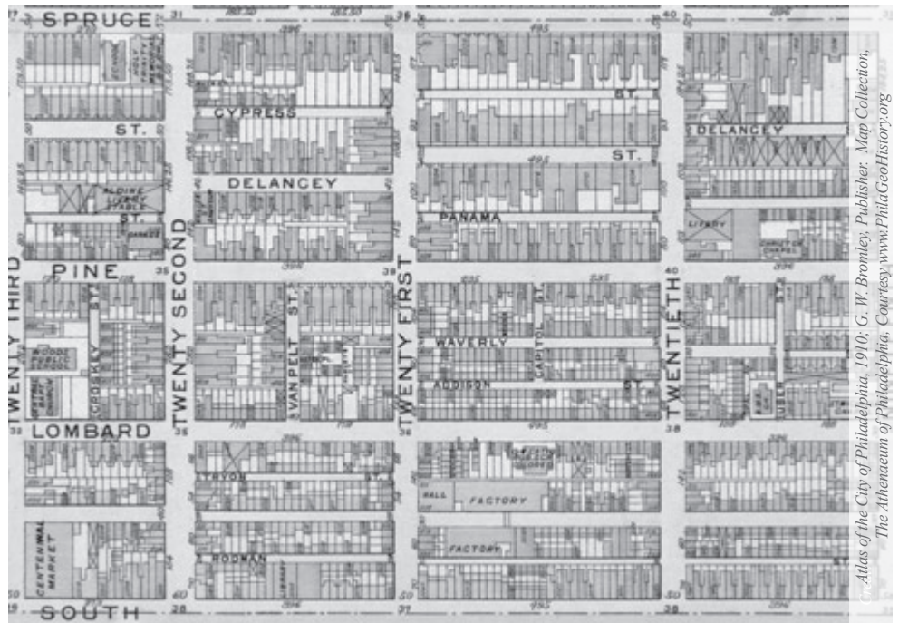
This 1910 "footprint" map showed lots but also included the footprint of the built properties allowing identification of changes to property footprints when maps from different years are compared.
