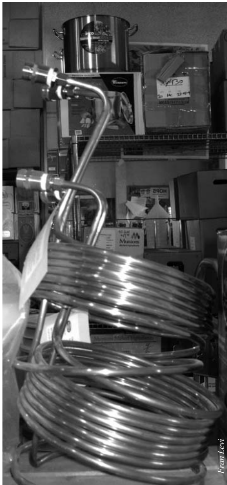
For sale at Home Sweet Homebrew is a copper WORT Chiller to rapidly chill brewed beer.
