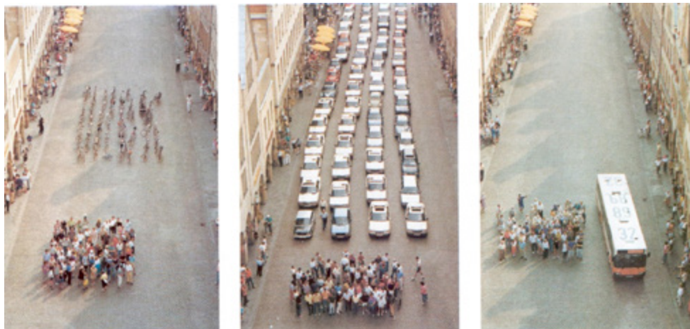
This triptych illustrates the relative numbers of vehicles—and the road space they occupy—needed to transport the same number of individuals, using bicycles, cars, and a bus, respectively.
